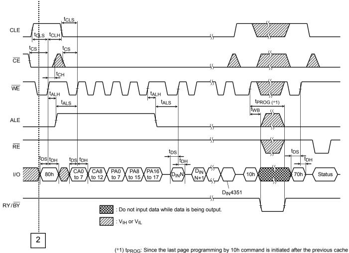
program, the t<sub>PROG</sub> during cache programming is given by the following equation.
