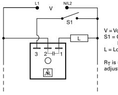
V = Voltage S1 = Optional Low Current Initiate Switch L = Load
