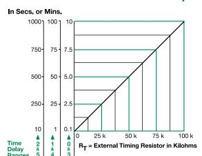
This chart applies to externally adjustable part numbers. The time delay is adjustable over the time delay range selected by varying the resistance across the  $R_T$  terminals; as the resistance increases the tie
