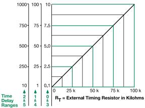
This chart applies to externally adjustable part numbers. The time delay is adjustable over the time delay range selected by varying the resistance across the R<sub>T</sub> terminals; as the resistance increases the tie
