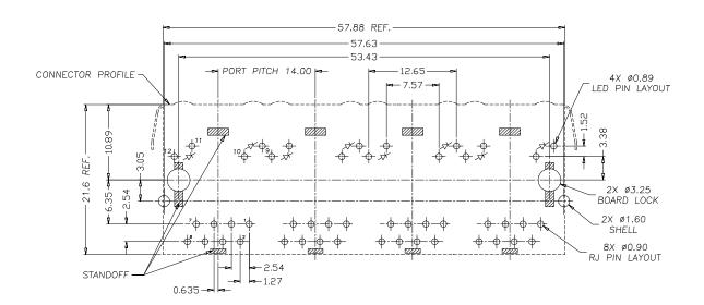
RECOMMENDED PCB LAYOUT  $\begin{array}{c} \hbox{COMPONENT SIDE} \\ \hbox{ALL DIMENSION TOLERANCE ARE $\pm 0.05 mm} \ \hbox{UNLESS OTHERWISE SPECIFIED} \end{array}$
