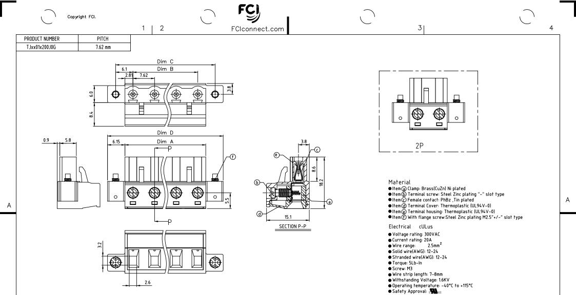
N = Number of poles Dim A=(N-1)X7.62+5.62Dim B=(N-1)x7.62
