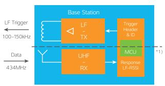
\*1) Graph shows one combined base station. Option is to split that as RX distance is much higher. So multiple trigger stations and one or few RX stations.
