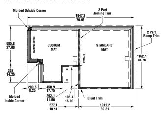
Step 3: When the Order is Placed, A Detailed Layout Showing all Components of the Trim System is Made
