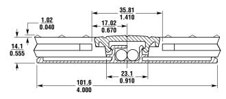
2-Part Joining Trim: PN 43222-0096 Joining Trim Aluminum Base: PN 32592 Joining Trim Cover Black: PN 32591 Joining Trim Cover Yellow: PN 32591-0010
