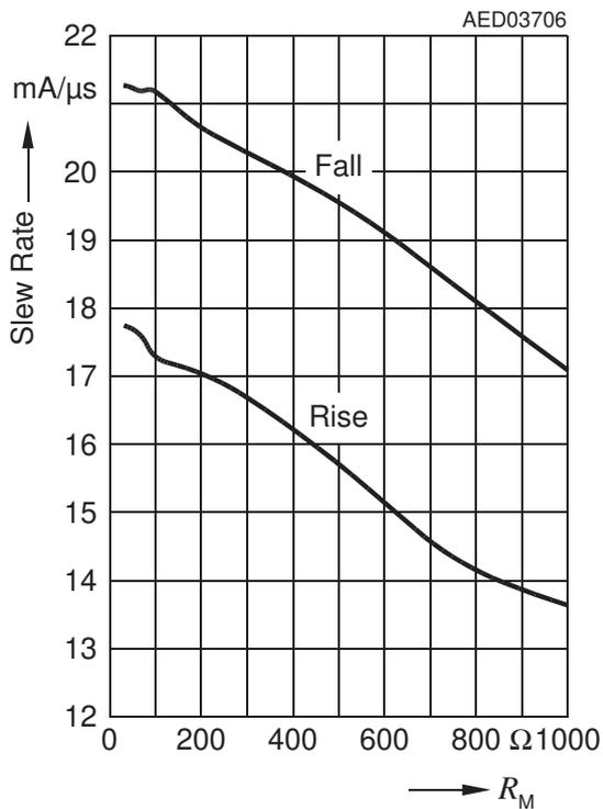
Slew Rate with  $C = 1.8 \text{ nF} = f(R_M)$
