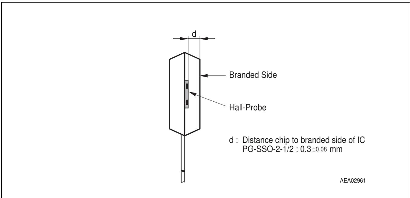
**Figure 12 Distance Chip to Upper Side of IC**
