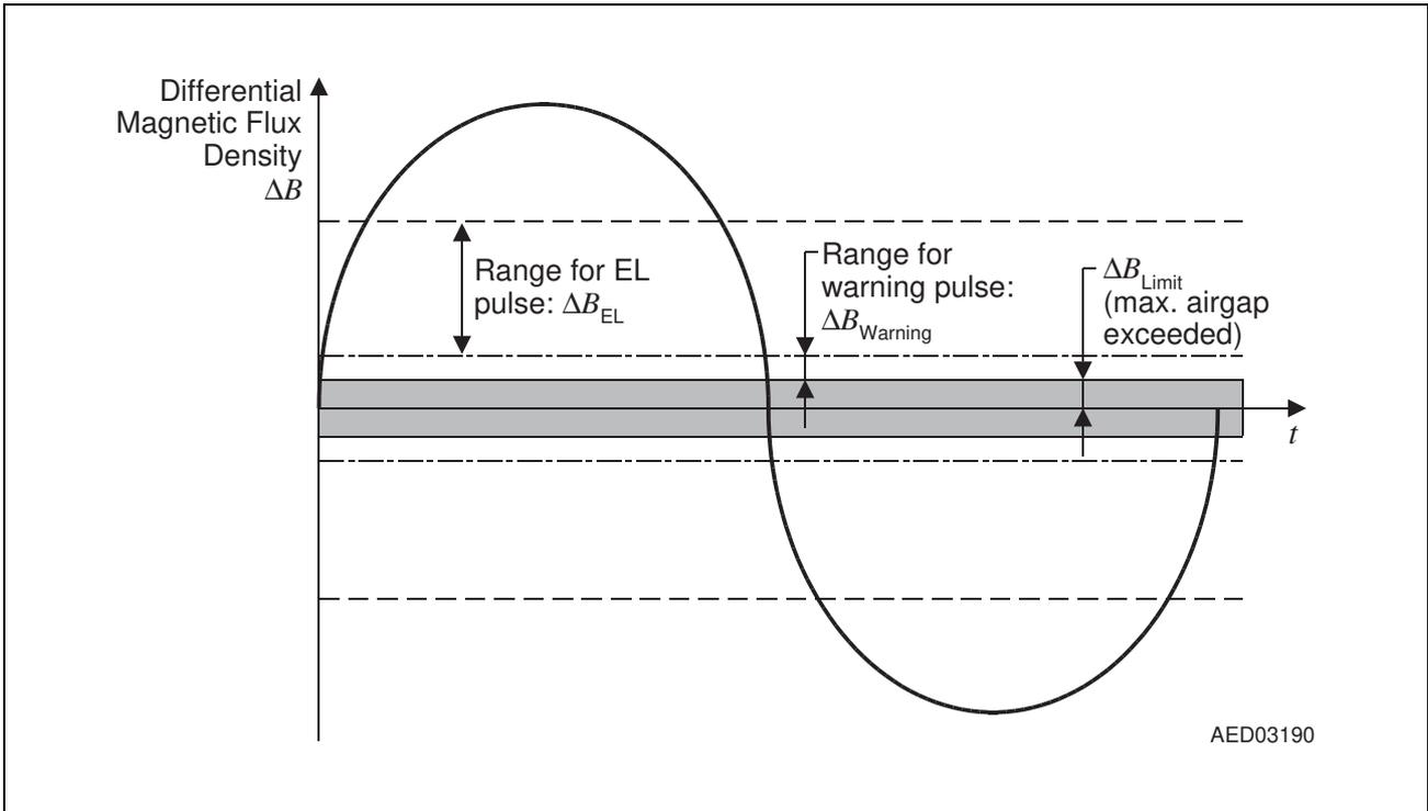
**Figure 4 Definition of Differential Magnetic Flux Density Ranges**
