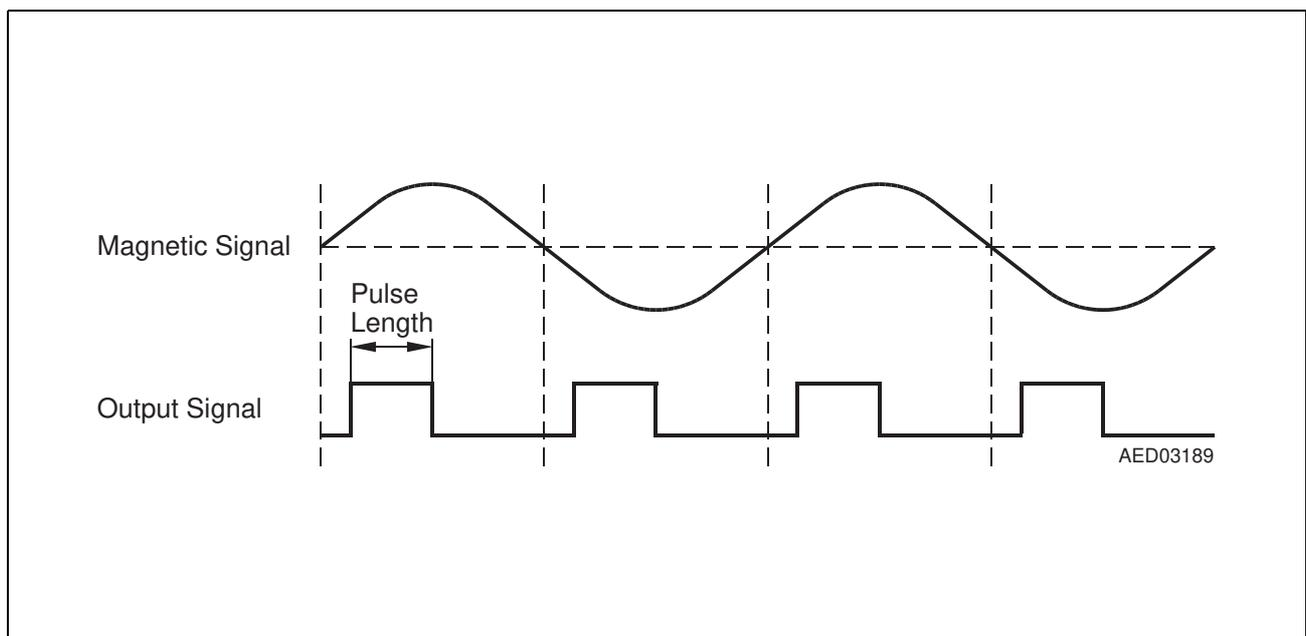
**Figure 3 Zero-Crossing Principle and Corresponding Output Pulses**
