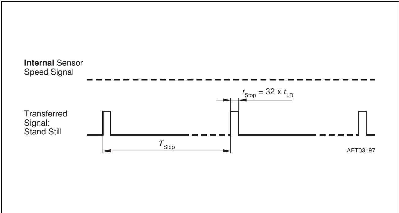
**Figure 9 Definition of Stand Still Output Pulse**
