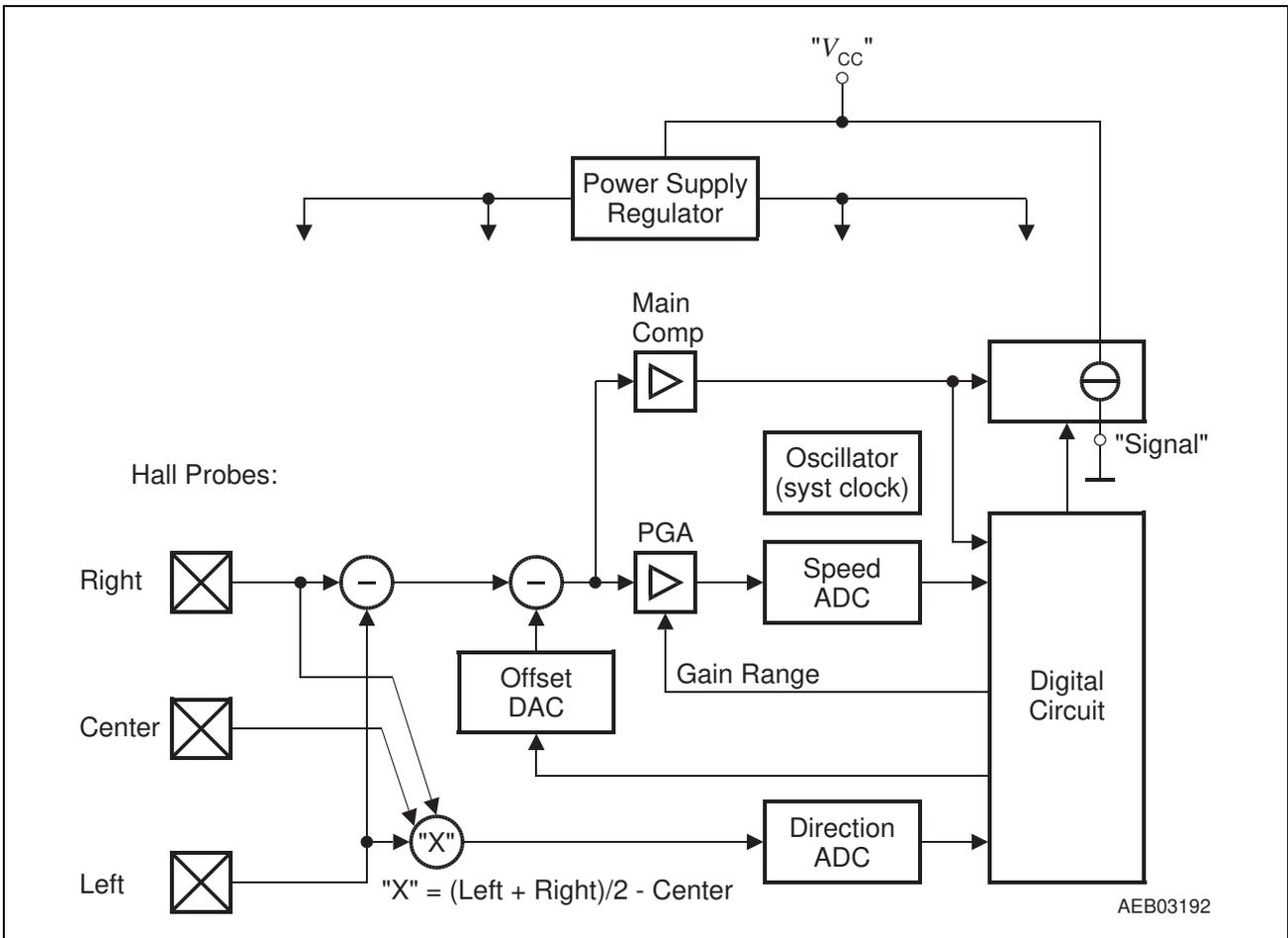
**Figure 2 Block Diagram**
