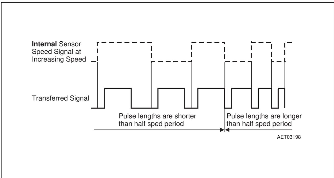
**Figure 10 Deviation of Duty Cycle at Fast Changing Frequencies**
