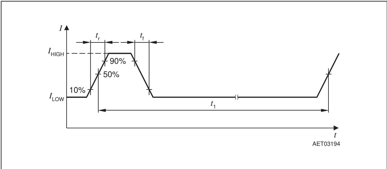
**Figure 6** Definition of Rise and Fall Time
