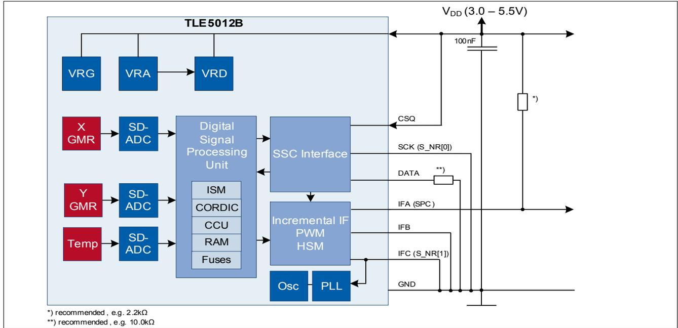
Figure 3-5 Application circuit for TLE5012B with only SPC interface (using internal CLK)
