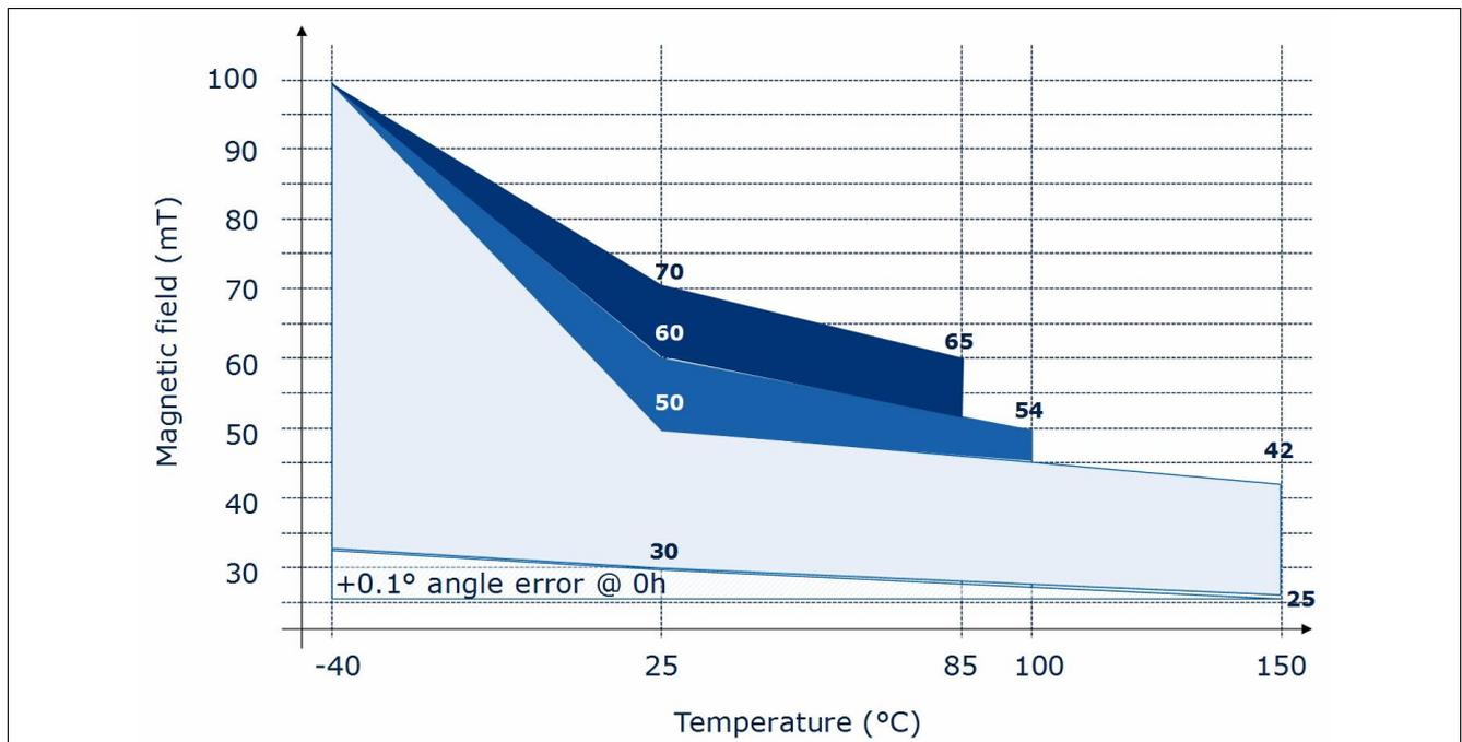
**Figure 4-1 Allowed magnetic field range as function of junction temperature.**
