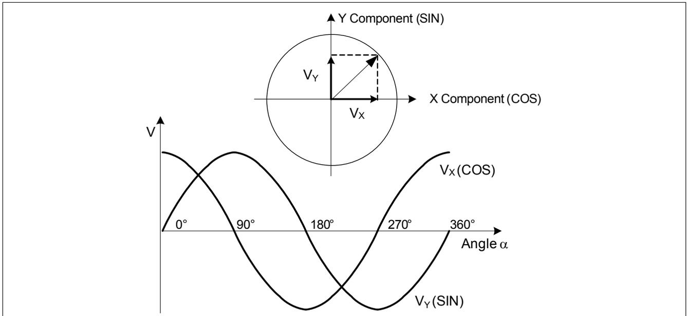
Figure 2-3 Ideal output of the GMR sensor bridges
