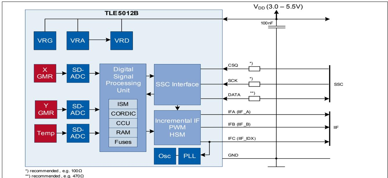
**Figure 3-1 Application circuit for TLE5012B with IIF interface and SSC (using internal CLK)**
