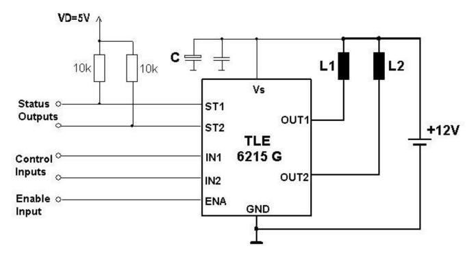
The blocking capacitor C is recommended to avoid critical negative voltage spikes on  $V_{\!\scriptscriptstyle S}$  in case of battery interruption during OFF-commutation.
