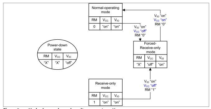
Figure 8 Mode changes by undervoltage events on V<sub>cc</sub>
