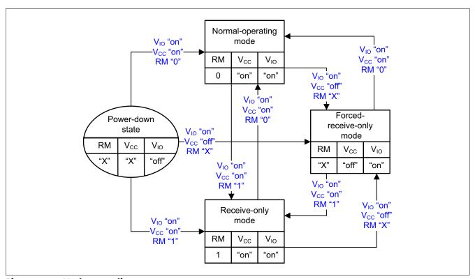
Figure 4 **Mode state diagram**
