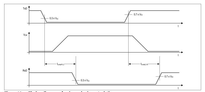
Figure 13 Timing diagrams for dynamic characteristics
