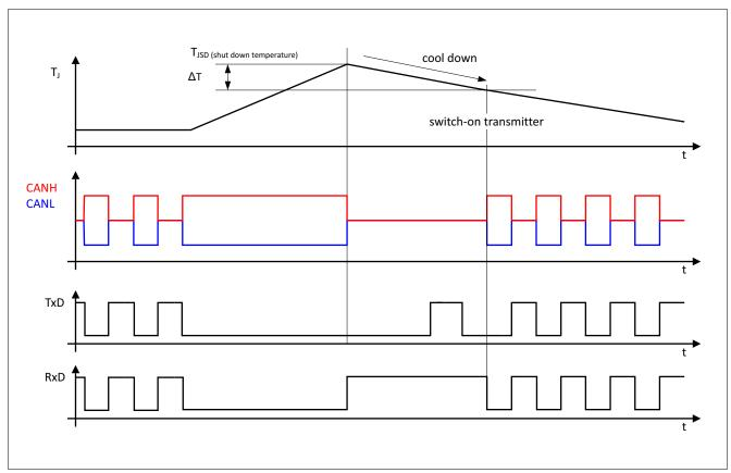
Figure 11 **Overtemperature protection**
