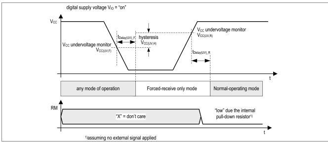
Figure 9 Undervoltage on the transmitter supply  $V_{cc}$
