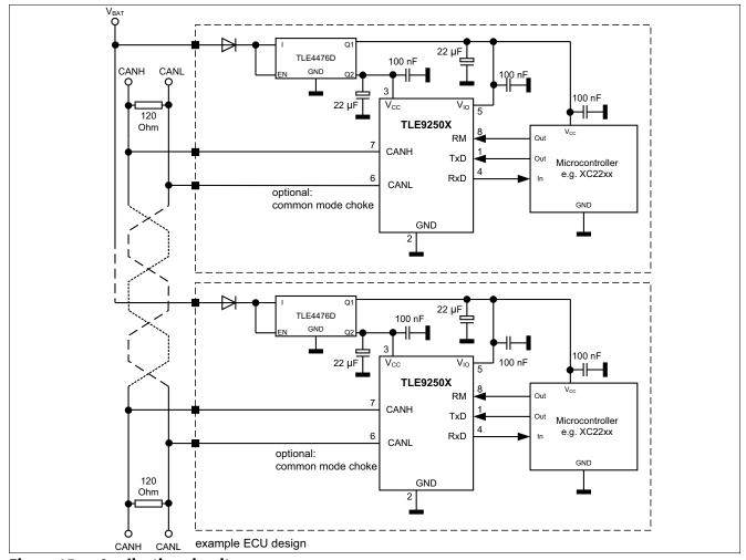
Figure 15 **Application circuit**
