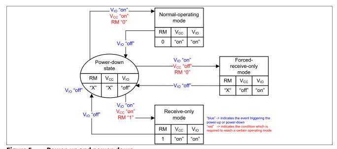
Figure 5 Power-up and power-down
