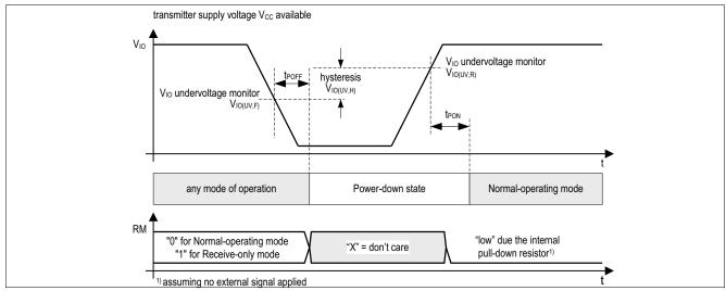
Figure 6 Power-up and power-down timings
