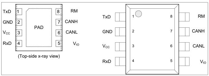
Figure 2 Pin configuration
