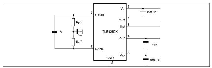
Figure 12 Test circuit for dynamic characteristics
