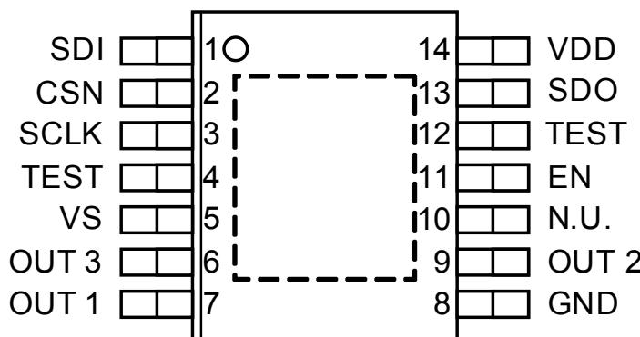
**Figure 1** Pin Configuration TLE94103EP with SPI interface
