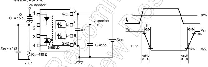
C<sub>L</sub> is capacitance of the probe and JIG. (P.G): Pulse Generator
