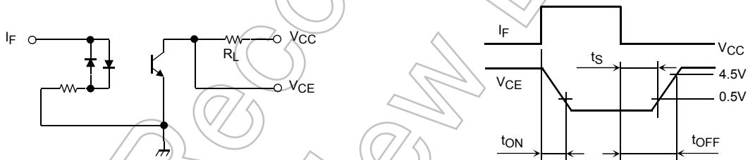
Fig. 1 Switching time test circuit
