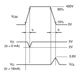
$$CM_{H}=\frac{320\left(V\right)}{t_{r}\left(\mu s\right)},CM_{L}=\frac{320\left(V\right)}{t_{f}\left(\mu s\right)}$$
