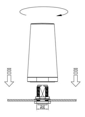
Recommended torque for mounting is 4.018 N.m or 41 kgf.cm Maximum torque for mounting is 9.8 N.m or 100 kgf.cm
