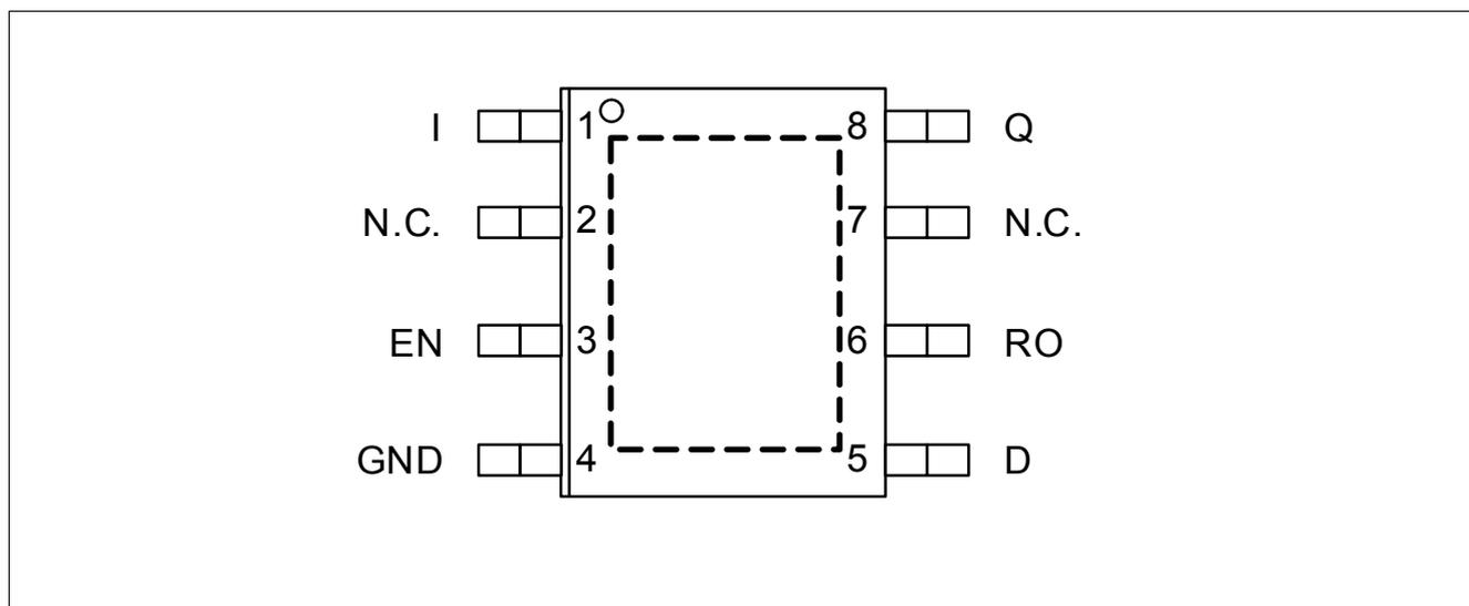
**Figure 2 Pin Configuration TLS810D1 in PG-DSO-8 EP package**
