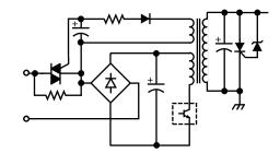
Two-phase motor control (for example, washing machine)
