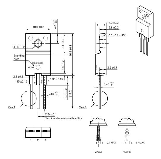
Gate burr: 0.3 mm (max.), mold flash may appear at opposite side Terminal core material: Cu Terminal treatment: Ni plating and Pb-free solder dip Leadform: 600
