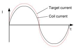
Coil current does not have optimum shape
