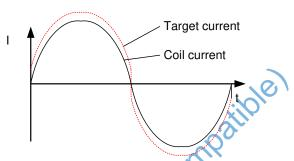
Coil current does not have optimum shape
