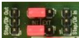
Figure 3.7 Jumper setting for TMC4210 selection.
