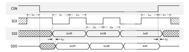
Figure 4.1 SPI timing
