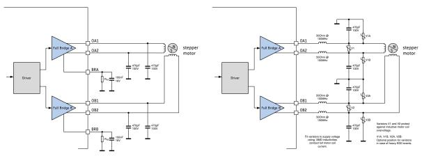
Figure 3.6 Simple ESD enhancement and more elaborate motor output protection
