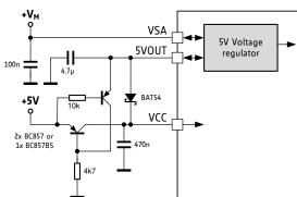
VCC supplied from external 5V using active switch. 5V or 3.3V IO voltage.
