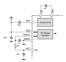
Figure 3.5 RC-Filter on VCC for reduced ripple
