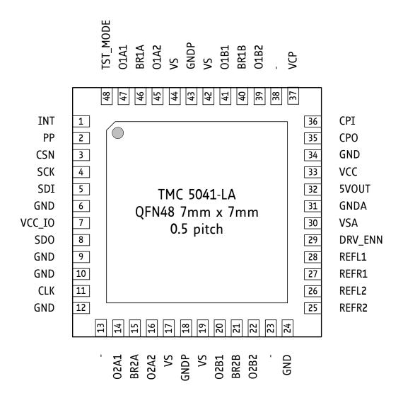
Figure 2.1 TMC5041 pin assignments.
