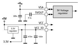
VCC supplied from external 5V. 5V or 3.3V IO voltage.
