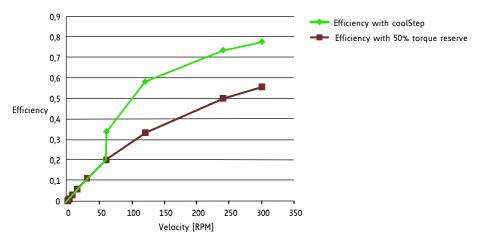
Figure 1.2 Energy efficiency with coolStep (example)
