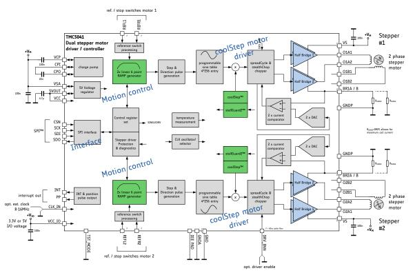
Figure 1.1 Basic application and block diagram
