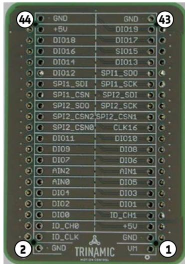
Figure 3.3 Eselsbrücke: pin assignment
