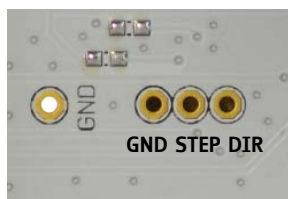
Figure 3.3 Test points for GND, REFL_STEP, and REFR_DIR
