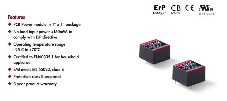
The TMPS-03 series are ultra compact AC/DC power supplies in a fully encapsulated plastic casing for PCB mount. Their safety approvals and extended operating temp. range from  $-25^{\circ}$ C to  $+70^{\circ}$ C qualify them for worldwide markets. They are certified to EN 60335-1 for household appliance and offer an interesting solution for space critical applications in commercial, and industrial electronic equipment and if compliance to ErP directive is required.
