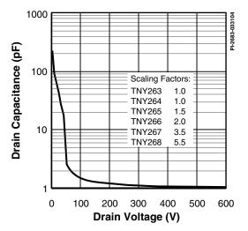
Figure 28.  $C_{\rm OSS}$  vs. Drain Voltage.
