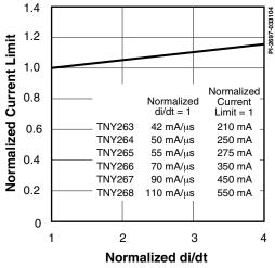
Figure 25. Current Limit vs. di/dt.
