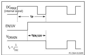
Figure 20. TinySwitch-II Output Enable Timing.
