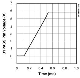
Figure 26. BYPASS Pin Start-up Waveform.
