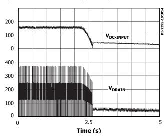
Figure 13. Slow Power-down Timing with Optional External (2 MΩ) UV Resistor Connected to EN/UV Pin.
