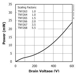
Figure 29. Drain Capacitance Power.
