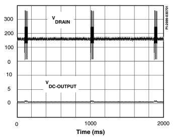
Figure 5. TinySwitch-II Auto-Restart Operation.
