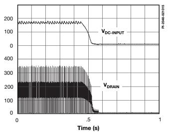
Figure 12. Normal Power-down Timing (without UV).
