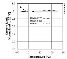
Figure 24. Current Limit vs. Temperature.
