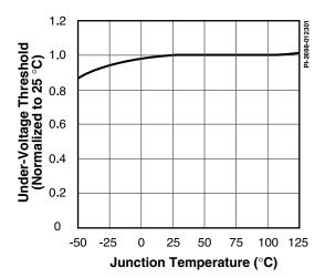
Figure 30. Under-voltage Threshold vs. Temperature.
