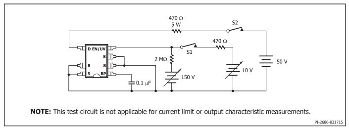
Figure 18. TinySwitch-II General Test Circuit.
