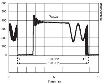
Figure 4. Frequency Jitter.
