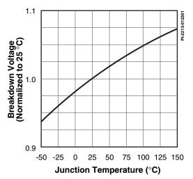
Figure 22. Breakdown vs. Temperature.
