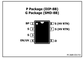
Figure 3. Pin Configuration.
