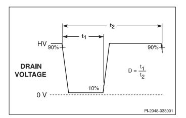
Figure 19. TinySwitch-II Duty Cycle Measurement.
