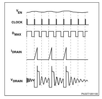
Figure 8. TinySwitch-II Operation at Medium Loading.
