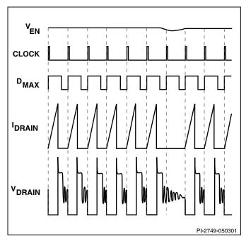
Figure 6. TinySwitch-II Operation at Near Maximum Loading.
