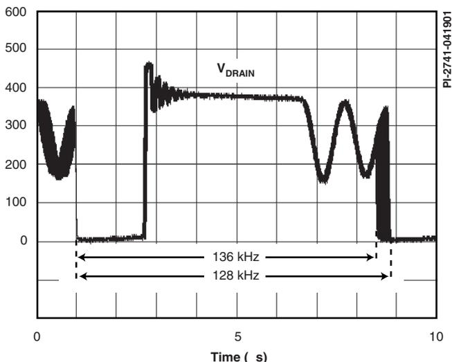
Figure 4. Frequency Jitter.
