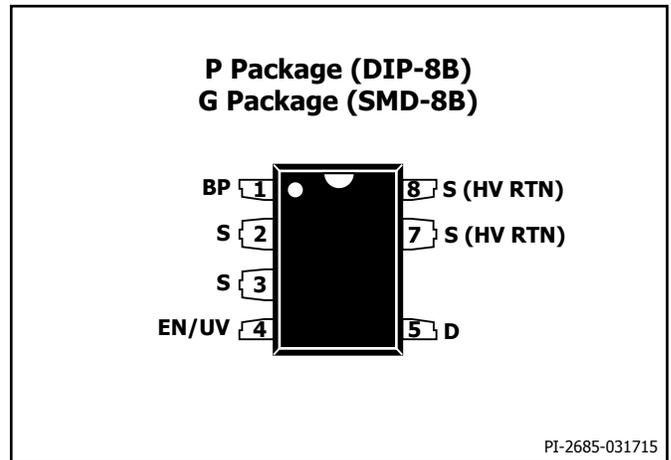
Figure 3. Pin Configuration.
