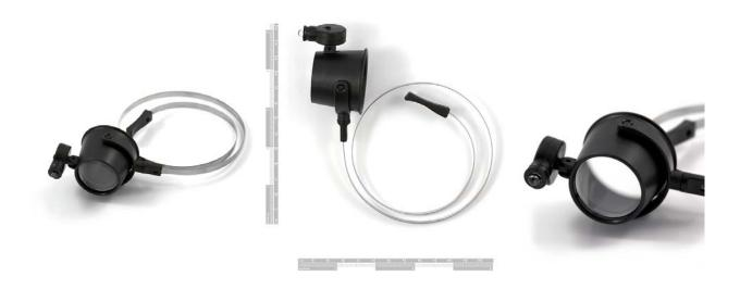
**Description:** When working with small parts, sometimes you need magnification and some extra light. This is a monocle we use regularly in our production facility. It has a 10x lens with a working distance of about 1-½". The 1" diameter eye piece fits snugly around your eye with a 15" aluminum-core headband. The LED provides sufficient light at the working distance.
