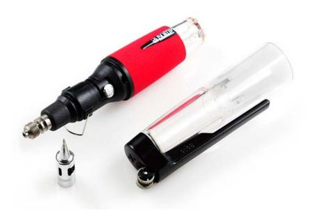
**Description:** The SolderPro 50 is an awesome little pocket-sized, butane-powered soldering iron. Soldering temperature is adjustable between 410-750?F. This thing is versatile too, with the torch tip you can use it as a soldering torch reaching a heat of up to 2400?F. They're ready to use quickly less than 20 seconds after ignition - and can run for up to 30 minutes on a single tank of butane.
