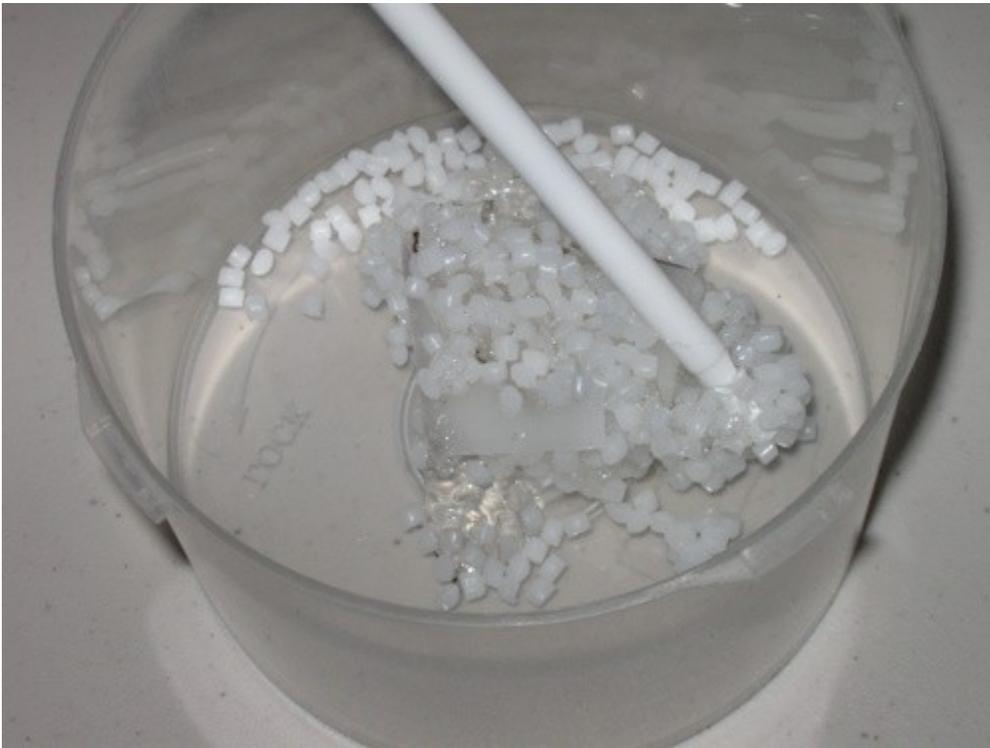
Granular polymer materials can be seen slowly melt into a liquid
