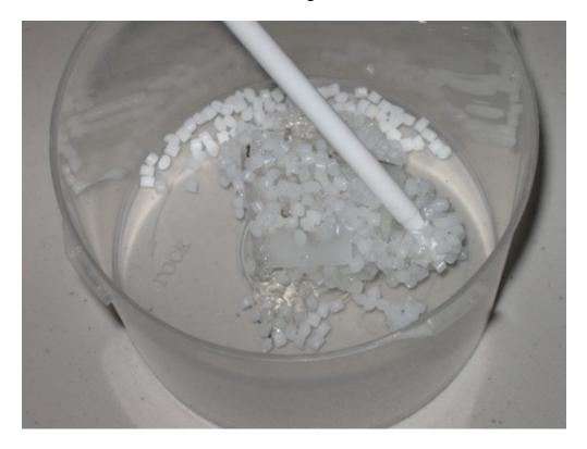
Granular polymer materials can be seen slowly melt into a liquid
