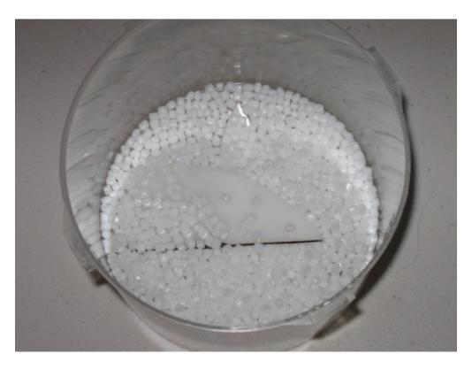
$65\sim90^{\circ}$  Add  $65\sim90^{\circ}$  C hot water mixing
