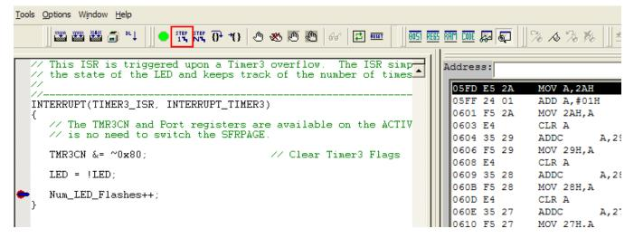
The disassembly window has three columns. The left column is the address of the instruction in Flash. The middle column is the instruction in hex. The right column is the disassembled instruction. The Disassembly debug window and the capability to single-step through firmware allows a developer to see exactly what instructions are executed and their output.
