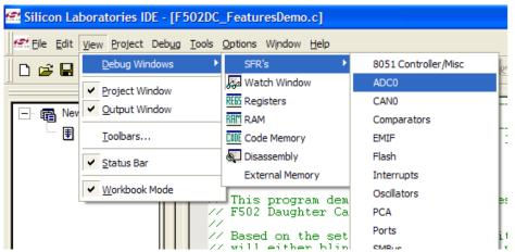
2. In the debug window, change the value of **ADCOCN** from 0x83 to 0x03. This value turns off the ADC on the target microcontroller.
