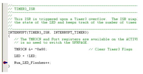
5. Start and stop the processor a few more times. Notice that the LED blinks once for every time the processor is started and the Num\_LED\_Flashes variable also increments by one.
