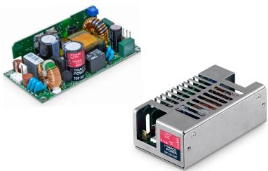
The new TOP-100 Series AC/DC Power Supplies feature the highest power rating in the industry standard 2.0"  $\times$  4.0" (50.8  $\times$  101.6 mm) footprint. They can supply up to 100 W output power with convection cooling over an industrial operating temperature range of -25°C to +50°C. This performance could be realized by a state of the art design providing an extremely high efficiency of >90 % which eliminates the need for a dedicated power supply cooling fan.
