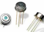
calibrated for temperature range up to 120°C or up to 200°C. The interrupt function also allows use of the sensor as a temperature alarm in industrial instrumentation.
