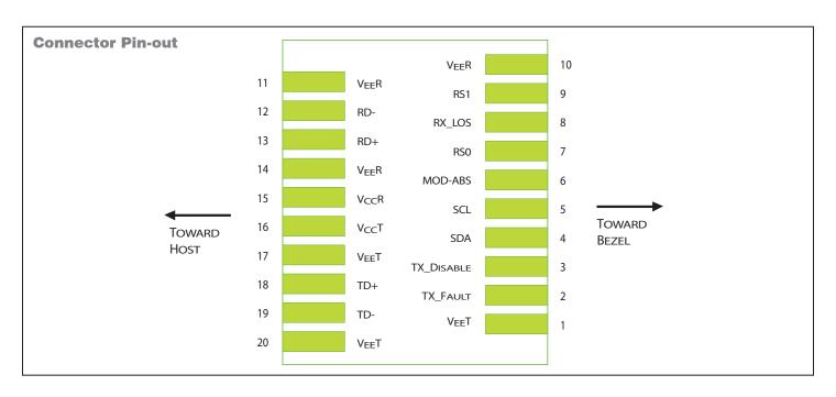
$<sup>^2</sup>$  Open collector compatible,  $4.7k\Omega$  to  $10k\Omega$  pull-up resistor to Vcc (Host Supply Voltage).
