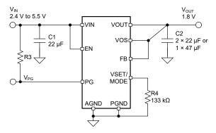
Figure 8-4. Fixed Output Voltage Application Circuit
