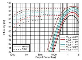
TPSM82866AA0HRDMR - Efficiency Versus Output Current; V<sub>IN</sub> = 5.0 V
