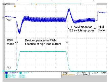
Figure 8-1. Optimized Transient Performance from PWM to PSM
