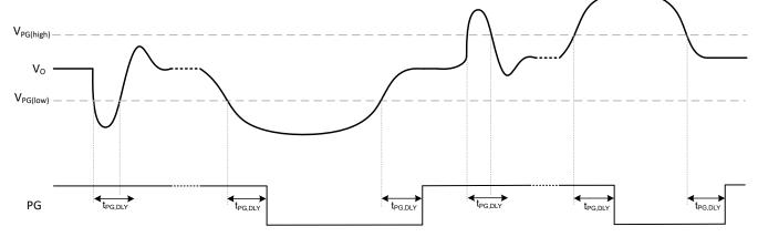
Figure 8-3. Power-Good Transient and Delay Behavior
