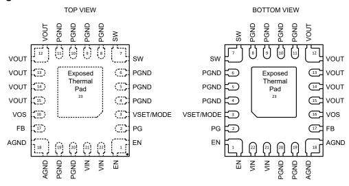
Figure 6-1. TPSM82864A, TPSM82866A - QFN (23 Pin)
