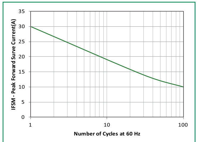
Figure 8 - Maximum Non-Repetitive Forward Surge Current Uni-Directional Only
