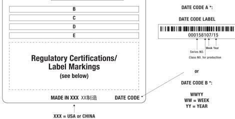
A=ITE / Medical Power Supply/Class 2/Household Power Supply B=P/N: (料号) TR9CB6667T00CIMR6B C=Model (型号) GTM96600-4005.9-T3 D=Input (输入) 100-240V~, 50-60Hz, 1.5A E=Output (输出)5.9 V --- 6.77 A ,40.0W
