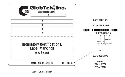
A=Medical/ITE/Household use Power Supply B=P/N: (料号) TR9KE3000T00-IMR6BG C=Model (型号) GTM96300-3614.5-2.5-T2 D=Input (输入) 100-240V~, 50-60 Hz, 1A E=Output (输出)12 V === 3.0 A ,36.0W
