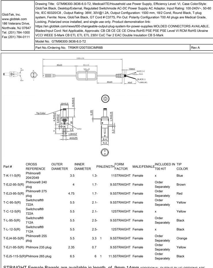
STRAIGHT Female Barrels are available in length of 9mm-14mm ADDITIONAL OUTPUT PLUG OPTIONS ARE AVAILABLE AT http://www.globtek.com/connectors/
