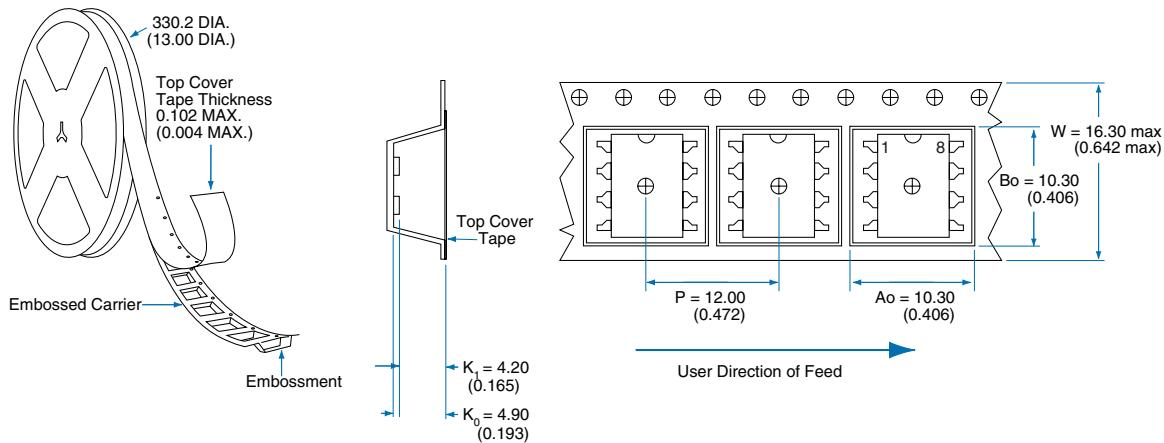
NOTE: Tape dimensions not shown, comply with JEDEC Standard EIA-481-2
