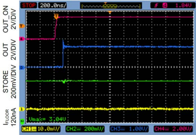
OUT_ON Switched ON : Circuit A with C OUT Removed V IN =1.2V, STORE=3V, I STORE =0.3μA, I OUT =3mA
