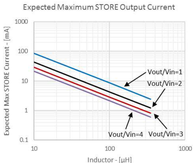
Figure 2.3. Expected Maximum STORE Output Current with 85% Efficiency vs. Inductor Value
