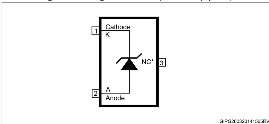
*Note:* The NC pin has to be connected to GND.
