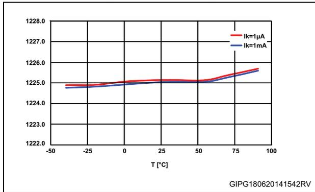
**Figure 3.  $V_K$  change vs temperature (1.25 V version)**
