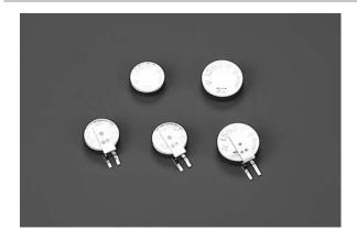
TS lithium rechargeable batteries are high capacity 1.5V type non-reflowable rechargeable batteries that provide sufficient discharge capacity with a charge voltage of less than 2.0V, and are intended for support of recent low-operating-voltage mobile devices.
