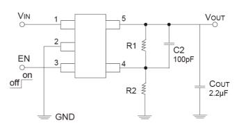
$V_{\text{OUT}} = 0.9 \; (\; 1 + \text{R1} \; / \; \text{R2} \; )$  C2 is unnecessary when R1 or R2 < 20K
