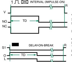
Digital integrated circuitry 1s - 1000m in 5 adjustable ranges or fixed ±0.5% or 20ms, whichever is greater
