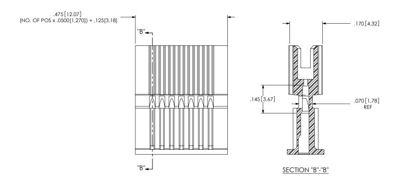
FIG 2 TFSD-07-S-S SHOWN (DIFFERENT AS SHOWN, OTHERWISE SAME AS FIG 1)
