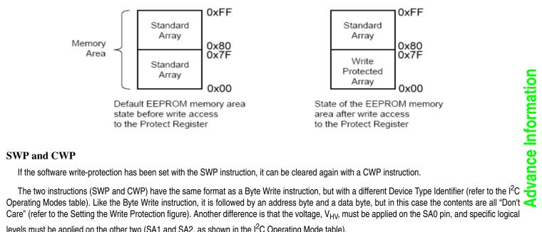
levels must be applied on the other two (SA1 and SA2, as shown in the I<sup>2</sup>C Operating Mode table).
